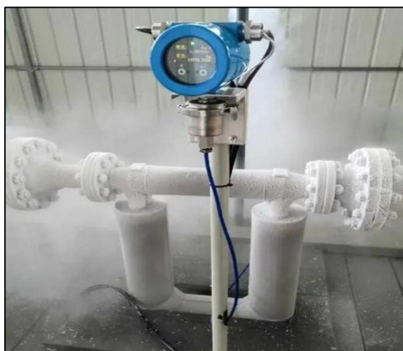
Figure 4: Experimental prototype of the proposed nitrogen level and flow measurement system.
