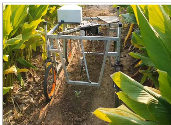
Figure 2: Prototype representation of the proposed robotic platform for weed detection and removal.
